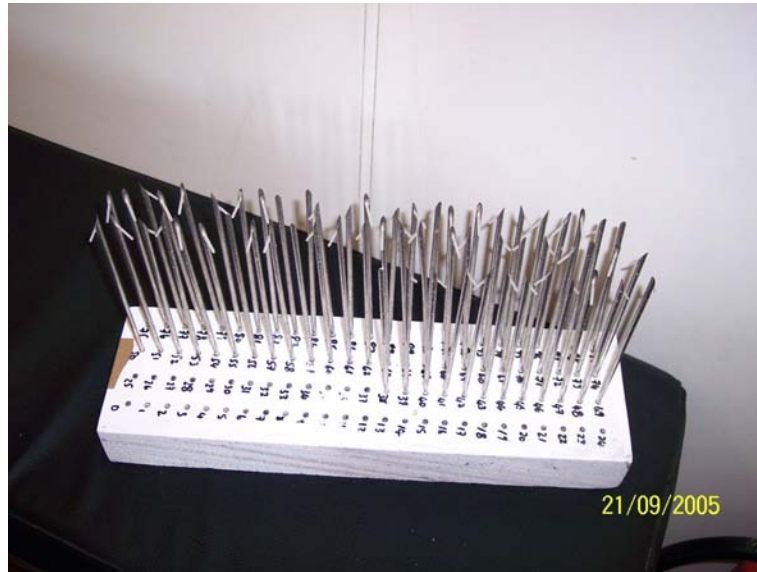
Plate 9: A tag holding block with dart tags already in applicators (Photo: R. Mugo).
