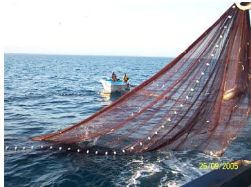
Plate 5: A seine net hauled by a hydraulic crane using a power block (Photo: R. Mugo).
